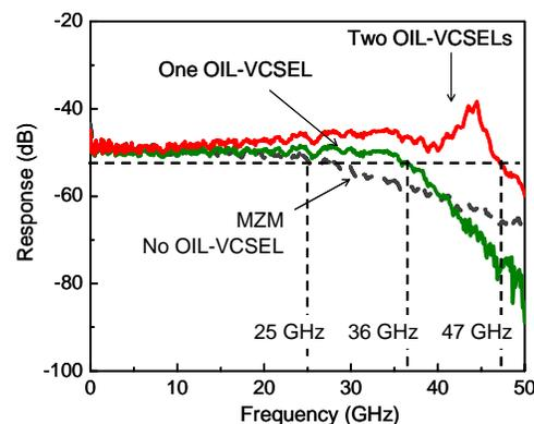
Fig. 3 Frequency response of the second scheme in Fig. 1 (b) where the signal is from external modulation of the master laser. Bandwidth of  $\sim 47$  GHz is achieved using two OIL-VCSELS.
