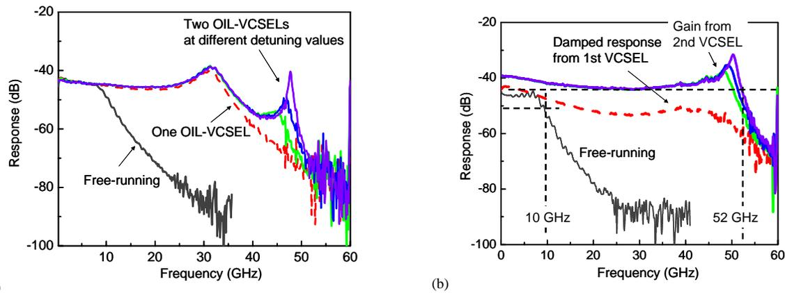
Fig. 2 Frequency response of the first scheme shown in Fig. 1 (a) where the first slave VCSEL is directly modulated. (a) peaked response showing the cascading effect (b) damped response tailored by adjusting the injection power and the detuning values of the two OIL-VCSELS.
