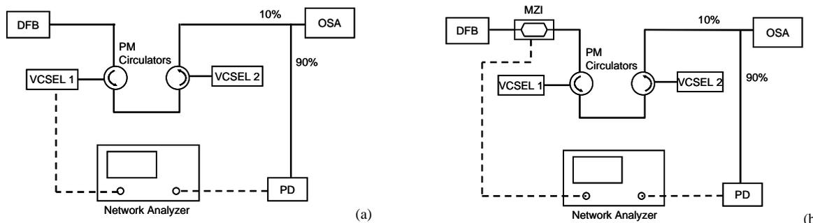
Fig. 1 Schematic of cascaded injection-locked VCSEL transmitters. (a) Modulation signal provided by the direct modulation on the first VCSEL (b) Modulation signal provided by the external modulation on the MZM (PM: polarization maintaining, PD: photodetector, OSA: optical spectrum analyser, MZM: Mach-Zehnder Modulator) Solid lines: optical path; dashed lines: electrical path
